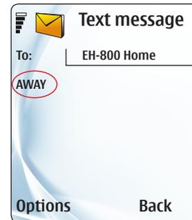
Use the away control command when you want to switch to a temperature drop. The controller maintains the temperature drop until it receives a "Home" control command. The control command can be given via a mobile phone, Home/Away switch or from the controller. If the controller has an exception calendar program in use and a "Home" control command has taken it from use, an "Away" control command will return the exception calendar back into use.
