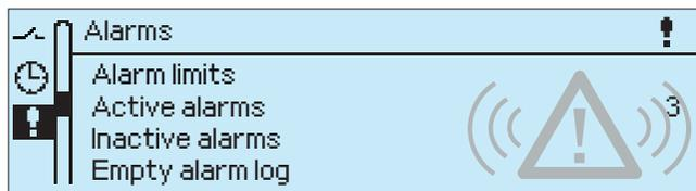
You can set alarm limits from the controller's alarm menu. Turn the control knob so the number is outside of the setting range to take the alarm out of use. The text "Not in use" will appear on the display. From the controller's alarm menu you can check the controller's active alarms and what alarms have been active. If the controller has active alarms, the number of active alarms will appear in the main alarm menu.
