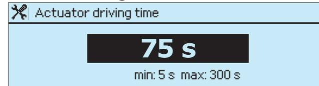
Give the actuator a run time. The run time indicates how many seconds go by if the actuator drives a valve nonstop from a closed position to an open position.
