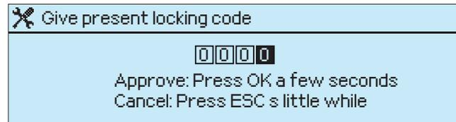
Write the new code on top of the old locking code.
