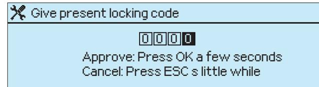
The controller asks for the present locking code. The locking code is 0000.
