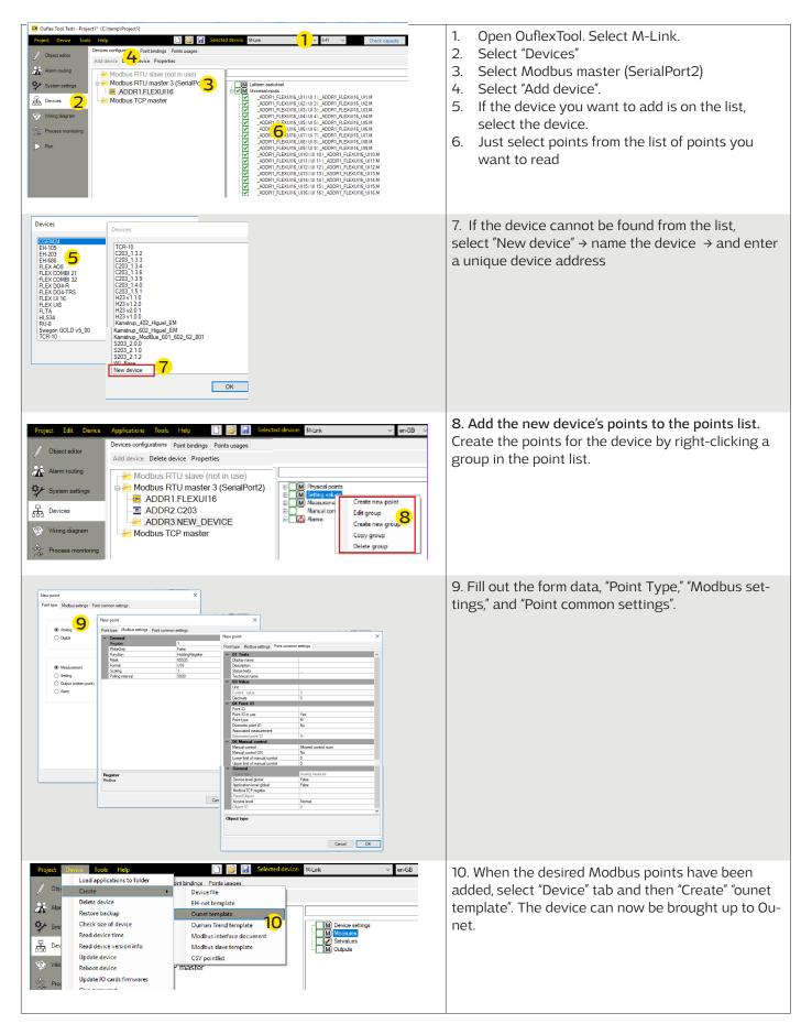
If you want Master devices to communicate with each other, connect the Master devices to the same subnet. This M-Link device works as a slave device. Modbus TCPIP server and client devices must have fixed IP.
