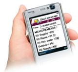
The controller sends B alarms to a GSM phone according to the clock program made here. The clock program principle is outlined on pages 14-15. In the example above, B alarms are transferred during work-days between 8:00 - 16:00. Note! In the event of a B alarm, the alarm relay can not be active if SMS transfer has been blocked.
