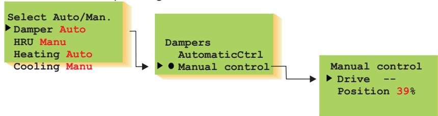
Note! When in the manual control mode the damper and cooling sequences go to 0-stage when the AH unit stops and return to the set manual control position when the AH unit starts up. When the AH unit is stopped the manual position % is 0. If it is not changed, the unit will run at the previously set manual control position when
