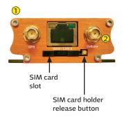
3G-MOD3 is delivered with the Ouman connection settings installed. If using the Ouman 3G-L1 or 3G-L2 connection, default settings can remain as set. If some other operator's SIM card is used, connection settings may need to be changed. For the correct data traffic settings, please contact your own service provider. To change connection settings, see the instructions on p. 2-4.
