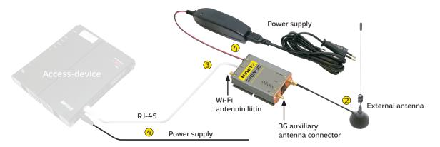
Ouman 3G-MOD3 is a 3G modem which can be used to create a mobile network in premises where such a network does not readily exist. Connection requires a SIM card with data connectivity (preferably with unrestricted data roaming. PIN code query must be disabled). The product package includes a 3G modem, power source and an antenna. SIM card with data connectivity can be acquired from Ouman (3G-L1 or 3G-L2) or your own operator.
