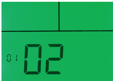
Image 3. OUMAN TCR-10 room unit is in programming mode.
