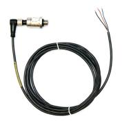
PX2.100P transducer can be use for measuring pressure of water, glycol or gas. The transmitter measurement area is 0... 6.8 bar (100 psi). Output signal is 0.25...10.25 V.
