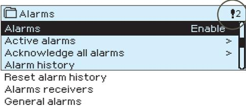
**H23 can send an alarm for a number of different reasons. Information about the alarm is shown on the display. The alarm also sounds a beeping noise.**
