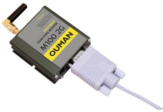
By connecting the modem to the H23 regulator, you can communicate with the regulator text messages and pass this information on alarms to your mobile via SMS.
