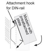
Use a DIN rail to fasten the modem into place. Attach the DIN rail to the wall. The modem has a preattached plate that can be attached to the DIN rail.
