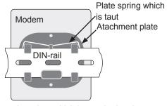
A modem which is attached to the wall, viewed from the back
