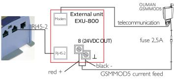
GSM modem power supply can be taken either online through the AC adapter or through the EXU-800 device connector number 8 (24 V OUT).
