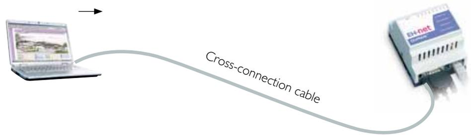
1. Connect the EH-net server to your computer using a cross-connection cable.
