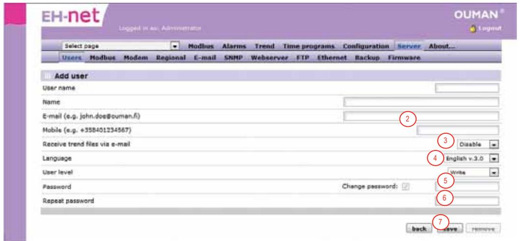
If the super administrator wants to receive alarms or test them in conjunction with configuration, the e-mail address and /or GSM number must be entered. (GSM modem must be connected to the EH-net)
