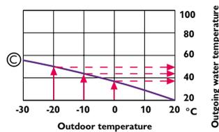
When it is  $-20^{\circ}\text{C}$ , the outgoing water is  $50^{\circ}\text{C}$
