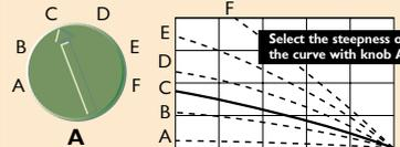
Curve C is selected in this example. If the room temperature goes down when the weather gets cold, select a steeper curve. If the room temperature goes up, select a lower curve. A suitable curve for your house may be between the plotted curves.
