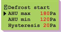
HRU defrost functions according to measurement information (Pa) from the pressure difference transmitter above the HRU, or according to switch information from the pressure switch.
