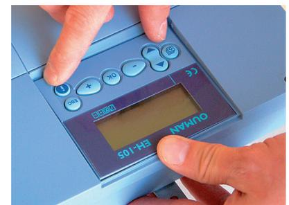
Press the keyboard/display unit carefully into place.
