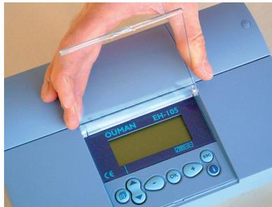
Remove the clear cover. Press as illustrated in the picture and pull the cover out of place.
