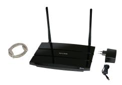
Access service can be used in places where the customer has an internet connection. Ouman devices, such as Ouflex, EH-Net and the EH-800 can be safely connected to the internet network by using the ACCESS service. Access device is added to an existing local area network. Access package includes an Access-device, RJ-45 cable and power supply. Access device can be connected to a local area network, in which
